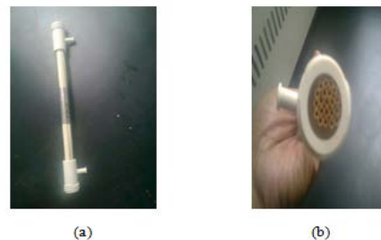
Fig 2. PVDF hollow fiber membrane module used in this research
